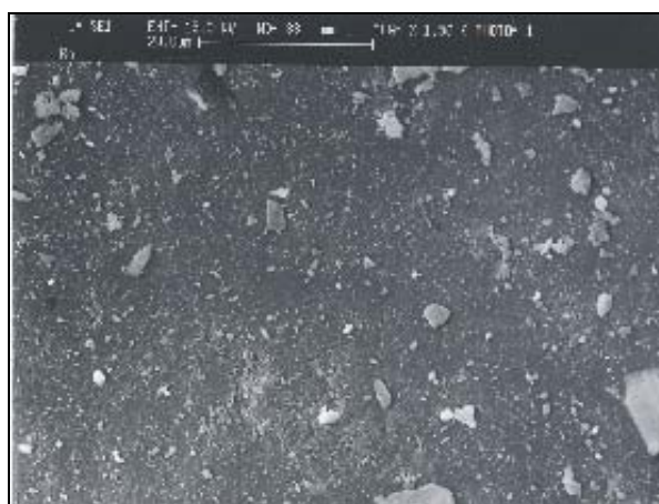
Figure 3.11 SEM micrograph of Pd-Co/SiO 2 at 20 X magnification
